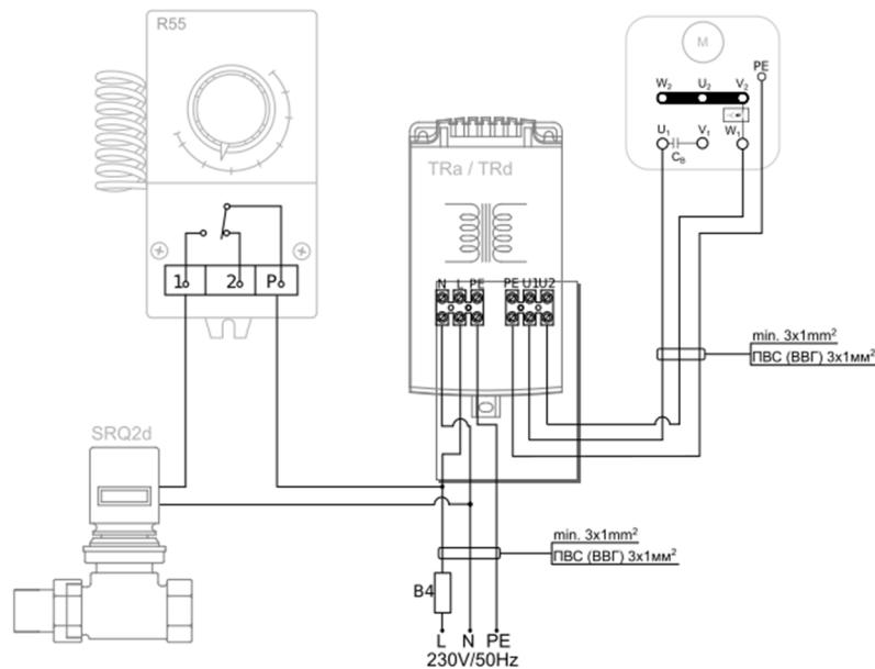
Thermostat R55 controls the operation of SRQ2d valve. TRa speed regulator allows for 5-step fan air flow switch.
