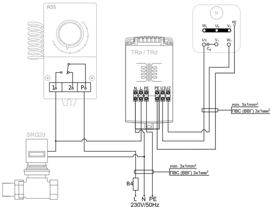
Thermostat R55 controls the operation of SRQ2d valve and TRa speed regulator. TRa allows for 5-step fan air flow switch.
